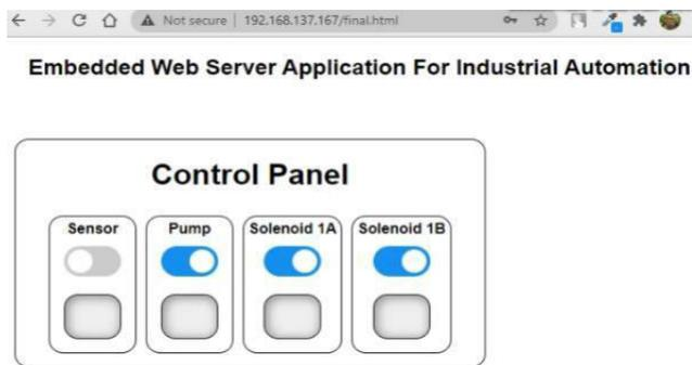
Fig. 9 Control Panel on Terminal Screen
